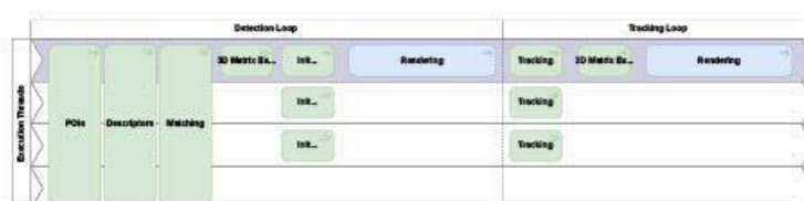
Fig. 4. Conceptual diagram illustrating the relative time each step consumes for the image based loops and if they are sequential, multi-threaded or asynchronous process. The highlighted lane represents the main thread of the application.
